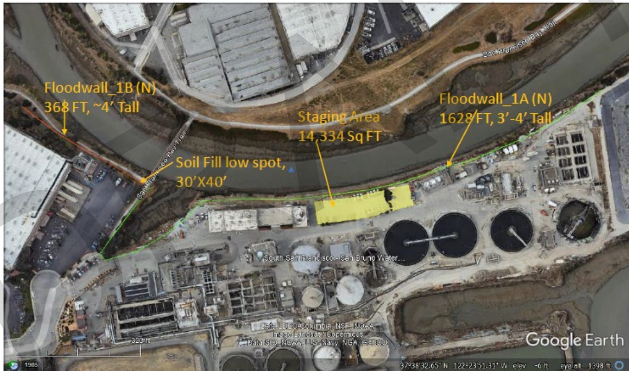
Figure 16. The floodwall on the North side of the WQCP is included in Alternatives 1 and 2, and would extend from the creek side of Costco, east to tie into higher elevation by the eastern side of the plant. The SF Bay Trail will not be impeded.
