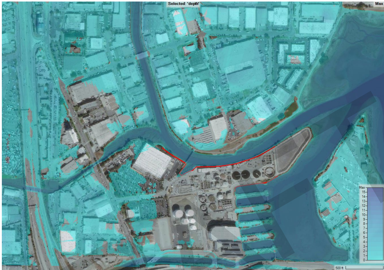
Figure 24. With-project floodwall alignments shown in red. Flood inundation resulting from a tidal event with maximum elevation of 12.65 ft, which exceeds the maximum elevation of 12.34 ft from a 0.2% ACE event with 50 years of intermediate sea level rise.
