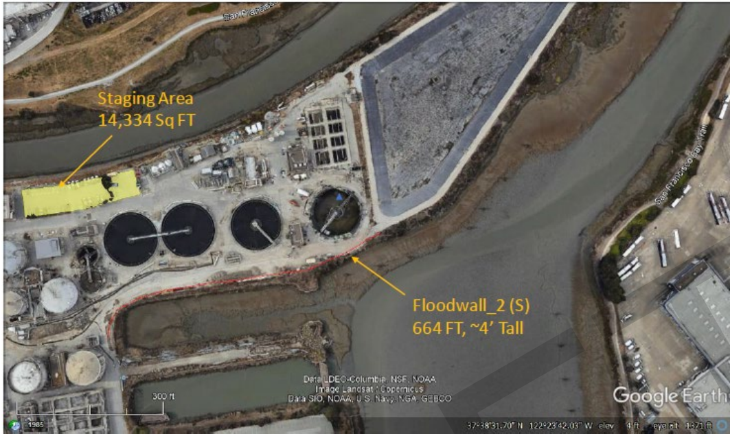
Figure 17. Alternative 2 also includes a shorter floodwall along the southern edge of the plant where elevations are lower, in addition to the north wall shown in Figure 4.
