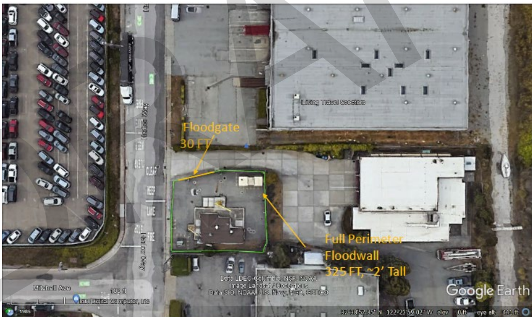
Figure 18. Alternatives 1, 2, and 3 all include a ring floodwall at sanitary pump station 4, which is roughly 2 feet high at grade, with a stop log gate which would need to be closed in a flood event to keep water out.
